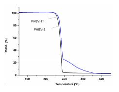
Fig. 8. TG thermogram of PHBV-S and PHBV-11.
